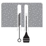
With the correct diameter drill bit, drill a hole to the correct depth (add at least 6mm to the depth to prevent the fastener from bottoming out).
