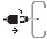
Attach the Hangerz® to the correct size socket driver and install anchor perpendicular to the base material substrate.
