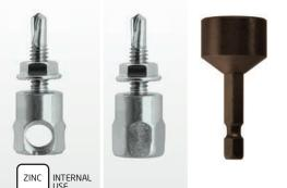
**ICCONS® Hangerz® for Steel** are a one-piece, high tensile self drilling fastening system suitable for installation into steel substrates. Hangerz® are ideal for suspending threaded rod vertically overhead for applications such as AC ducting, hanging pipe, fire protection, and cable-tray applications.
